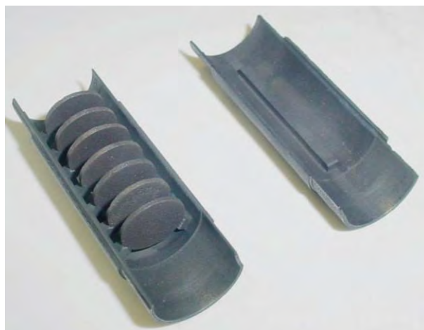
Figure 1: A uranium carbide target prototype used for irradiation tests.
