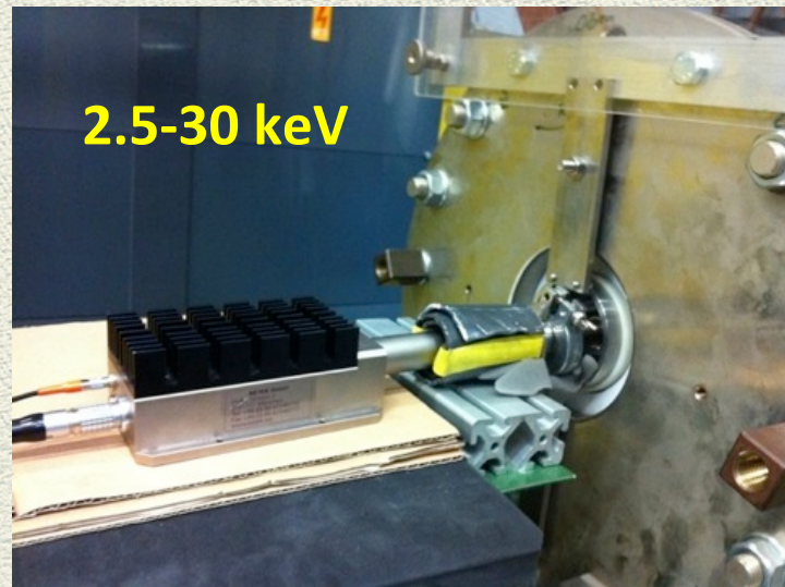
SDD detector for warm electron component
